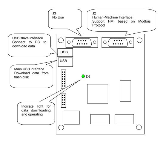
J2: HMI (RS232) -support HMIs such as EasyView, BYDseries HMI, PAD03, etc. based on Modbus Protocol
