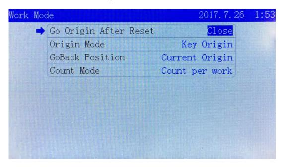
Move the cursor to  $\llbracket$  Go Origin After Rest  $\rrbracket$  and press  $\llbracket \leftarrow \rrbracket$   $\rrbracket$  . You can choose "back to origin point after a reset" as on or off.
