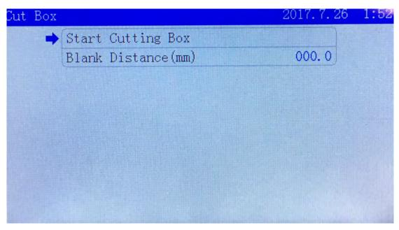
• Blank Distance(mm): The distance from File Box position to the actual cutting box position.
