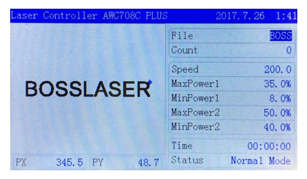
Pressing 【Enter】 a second time to enter the file parameter settings. Move the cursor to 【Document Params Settings】, Press【Enter】 to enter the document parameters settings as shown below.
